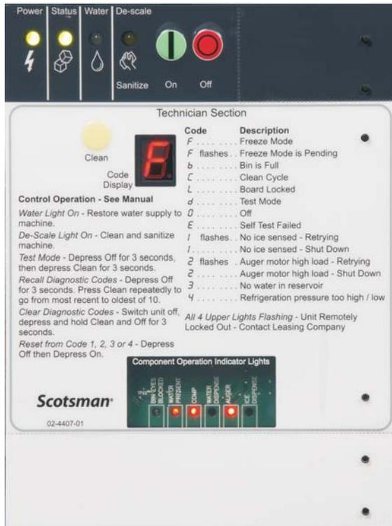
At the beginning of any restart the controller will display a blinking F.
