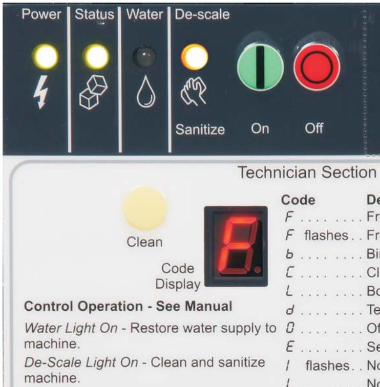
After 6 months of power up time, the De-Scale & Sanitize light will be switched On. It will switch off after the machine has been through a cleaning process, as described here:
