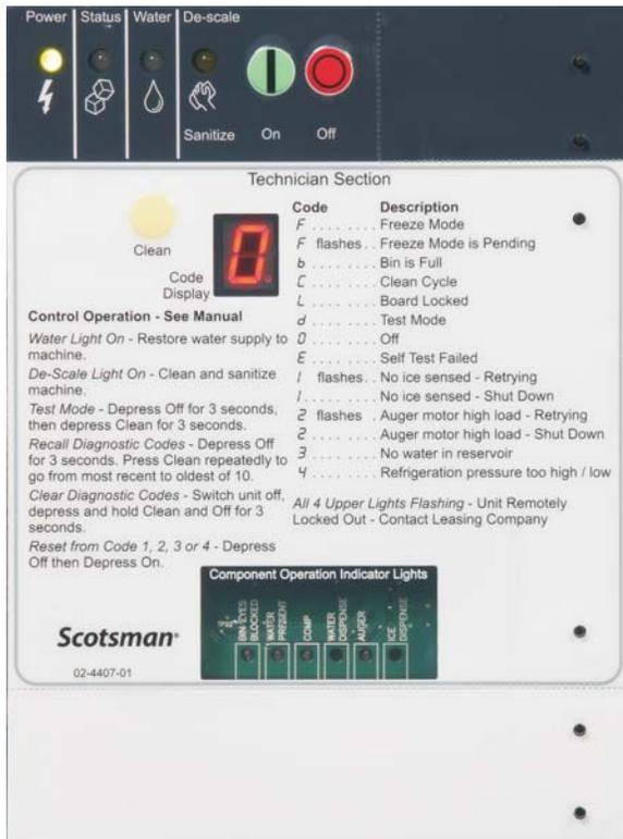
When power is supplied, the four lights at the top and the display indicator will blink on and off one time. Then the Power light will be on and a 0 is displayed.
